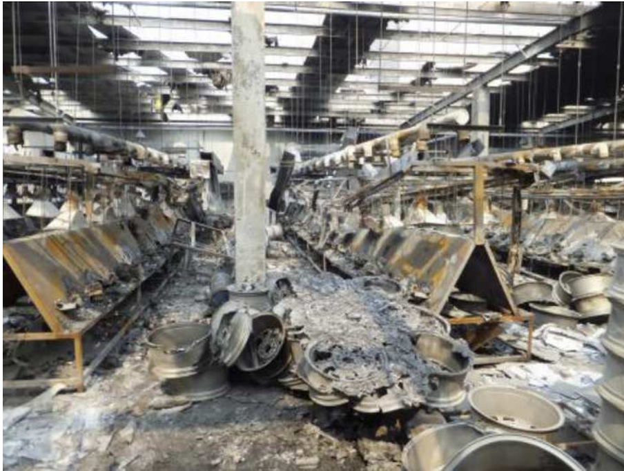
Figure 1.1: Destroyed polishing production lines after an aluminum-alloy dust explosion catastrophes in Kunshan, China, 2014 [2].
