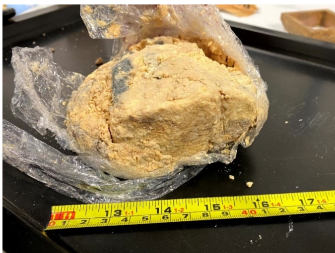
Figure 25: KSL_13 turned out very brittle and remarkably light weight (27.09.2022).
