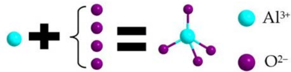
Figure 2-12: Schematic of the formation of tetrahedral aluminate units. [9]
