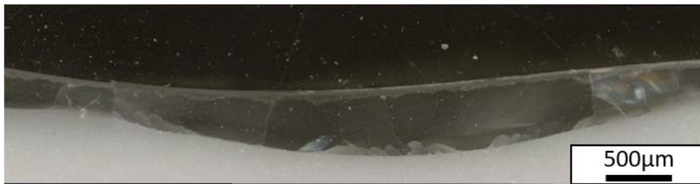
Figure 6-1: Attack on Al 2 O 3 crucible (white) from interaction with slag N3.
