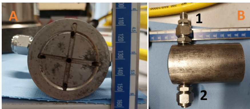
Figure 4-8: A: Contact surface of the in- & outlet stamp. B: Height of the in- & outlet stamp. 1 = Connection for stainless-steel line; 2 = Blind cap to ensure tightness.
