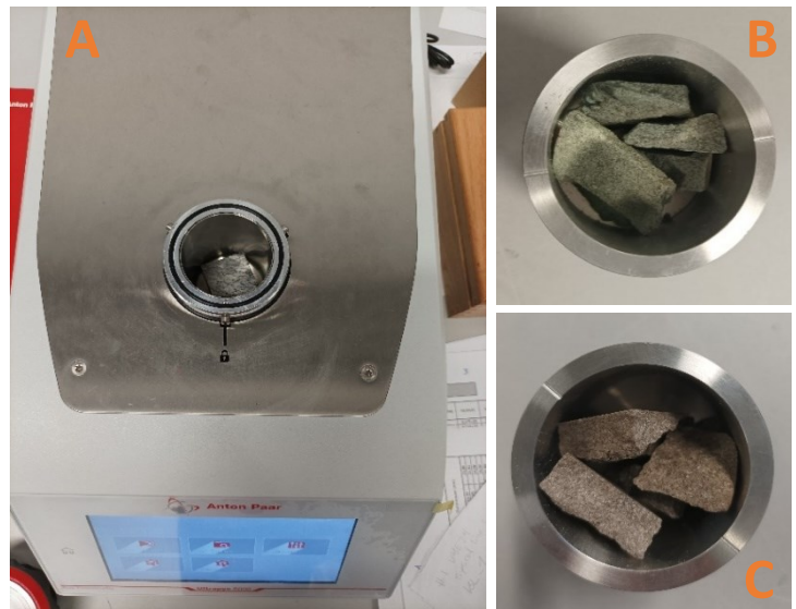
Figure 4-4: A: Top view of the gas pycnometer Ultrapyc 5000 from Anton Paar. B: Sample chamber filled with the Trattnach sandstone. C: Sample chamber filled with the Ruhrsandstone.
