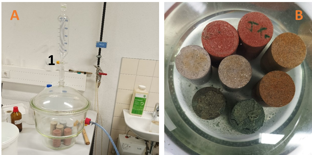
Figure 4-3: A: Creation of vacuum before adding distilled water. 1 = stopcock. B: Desiccator filled with distilled water and rock samples.
