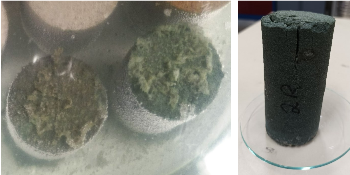
Figure 6-1: A: Organic material is extracted during the water saturation method. B: Visible mechanical damage of sample 2R after the experiments.
