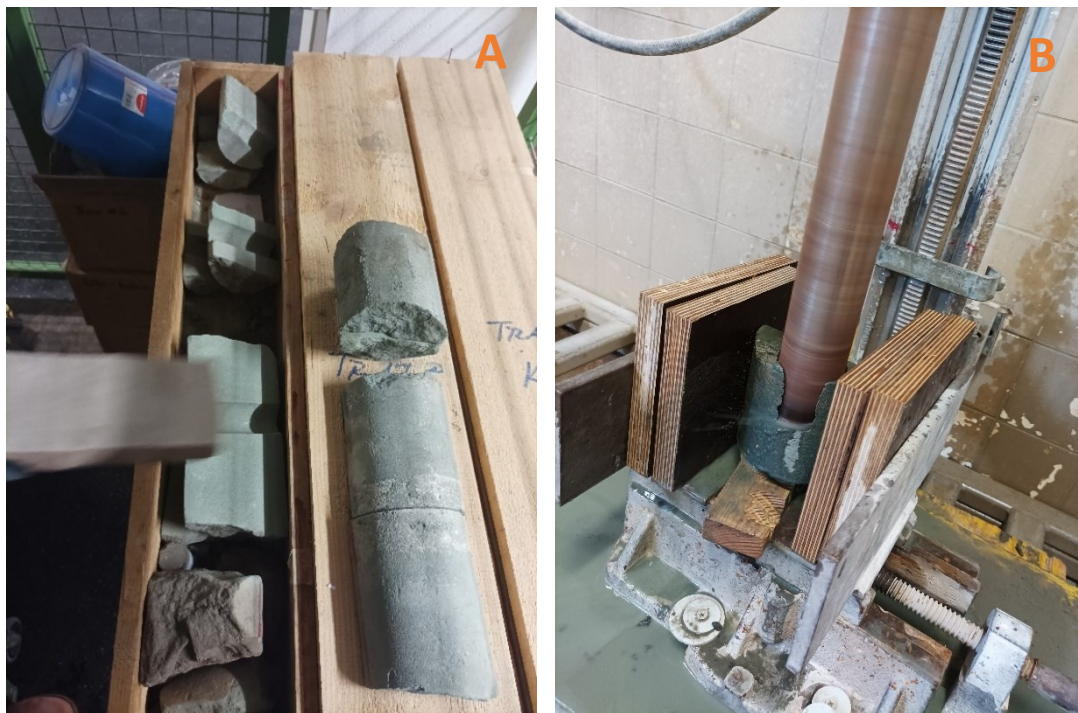
Figure 4-1: A: Drill core of the Trattnach oil field by RAG Austria AG depth 1600m. B: Drilling procedure to obtain a cylindrical shaped sample with an approximate 2:1 length to width ratio.
