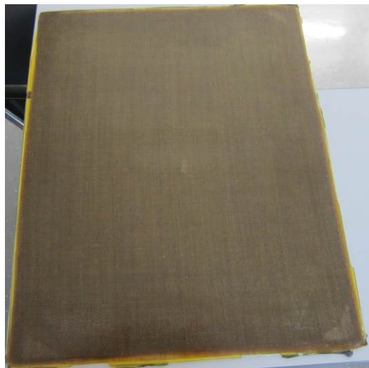
Figure 5: Manufactured plate by Pressing Moulding
