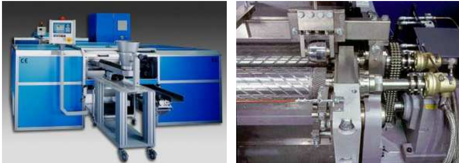
Fig. 4. Shear rolls for continuous production of feedstock materials (courtesy of Bellaform GmbH, Germany, www.bellaform.com ).
