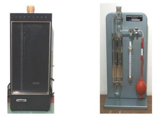
Figure 18: Photographs of the Permaran Outokumpu (left); and the Blaine apparatus manufactured by Tonindustrie Prüftechnik (right)
