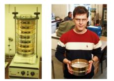
Figure 17: Prescreening on a test sieve shaker, completed by manual screening
