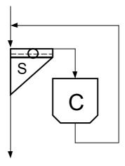
Figure 1: Scheme of the closed circuit design with prescreening. S ... screening, C ... comminution
