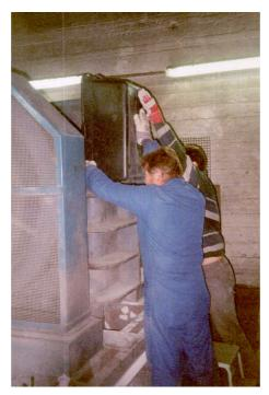
Figure 14: Feeding the crusher
