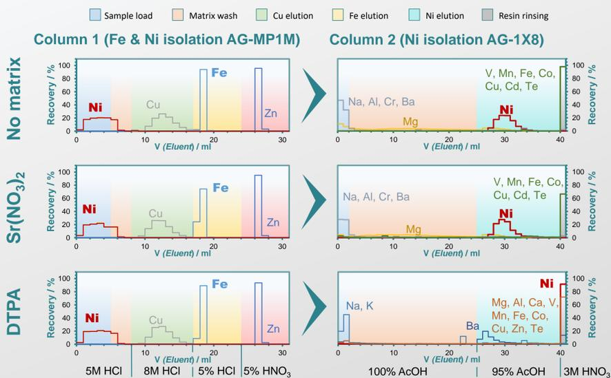
Fig.4: Elution profiles for Fe and Ni separation using AG-MP1M and AG-1X8 resins for different matrices typical for soil extracts
