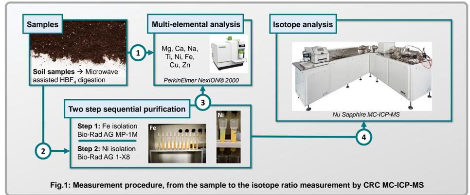
Fig.1: Measurement procedure, from the sample to the isotope ratio measurement by CRC MC-ICP-MS
