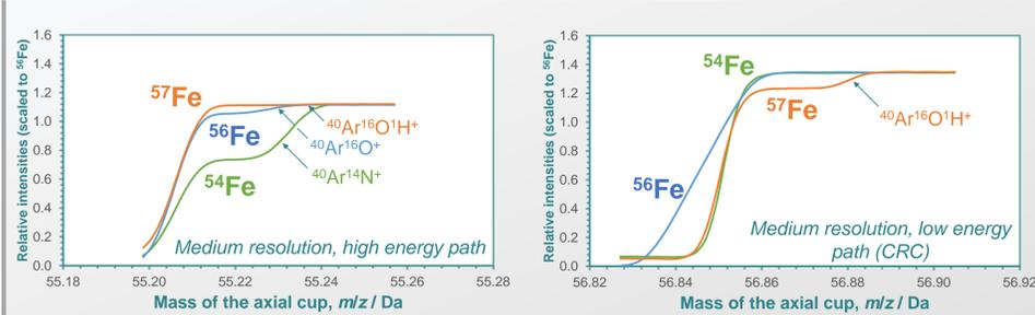
Fig.3: Magnet scans observed for Fe isotopes ( $w = 100 \text{ ng} \cdot \text{g}^{-1}$ ) and their interferences in medium resolution with and without CRC
