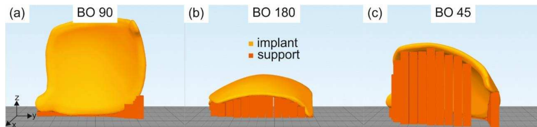
Fig. 1: The three different build orientations (BO) of the PSCIs displayed in the slicer software.
