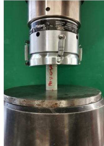
Figure 8: UCS testing apparatus with rock sample during loading.
