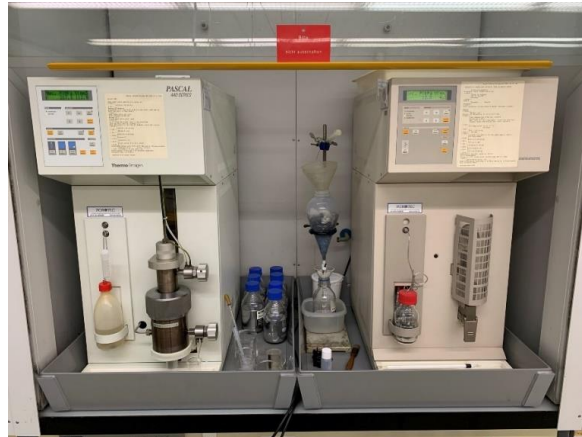
Figure 11: Low- and high-pressure chambers to analyse porosity and pore size distribution. Right: low-pressure device for mercury intrusion, left: high-pressure device to further induce the mercury into nanometer pores using high-pressure
