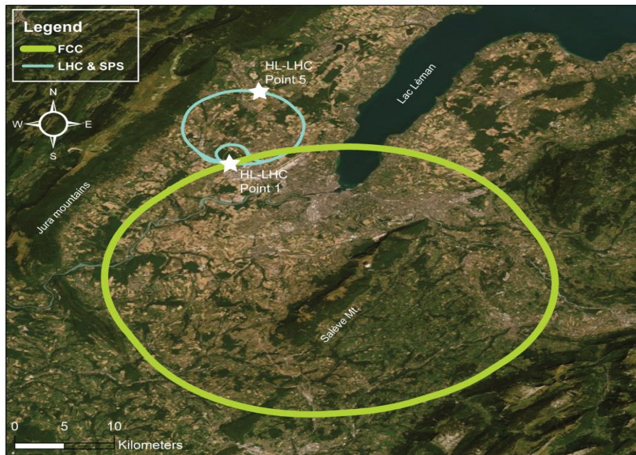
Fig. 1 The FCC ring layout in green with the LHC (large) and its predecessors (small) both in blue.
