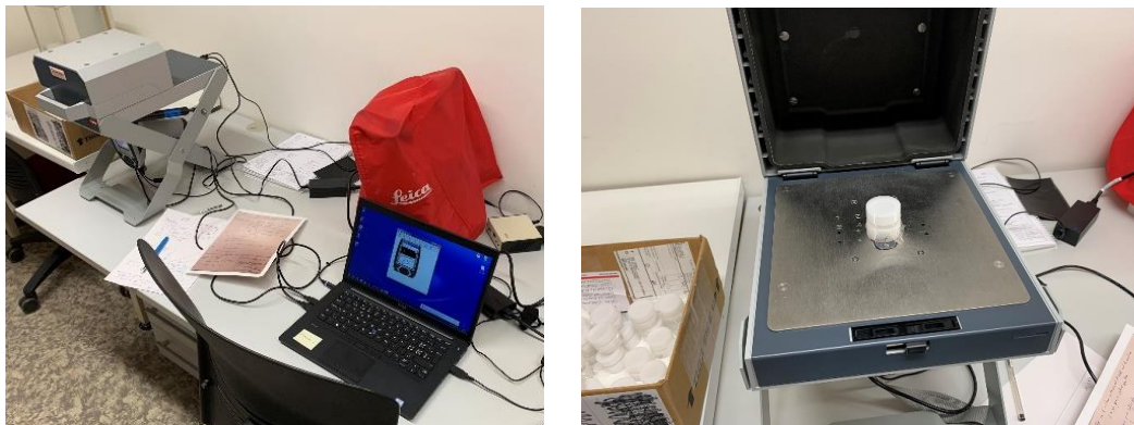
Figure 4: Left: Measuring pXRF device with electronic equipment and laptop for machine controls and data processing, right: close-up of portable XRF device with powder sample on beam hole when device is turned off. pXRF can be directly used on outcrops or core samples with lesser precision than with powder on the desk system but with higher efficiency. This makes it a good measuring device also at the tunnel face or in a truck.
