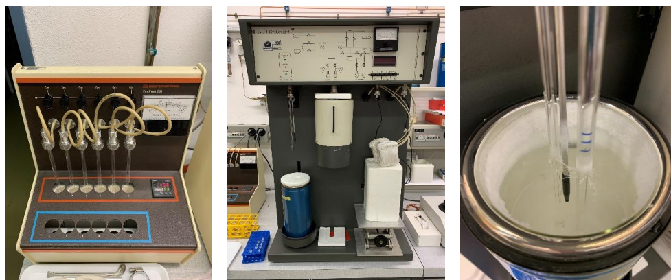
Figure 8: Left: VacPrep 061 vacuum pump used for sample degassing, middle: Quantachrome Autosorb-1 device for measuring specific (outer) surface, right: close-up of liquid nitrogen tank, in which sample is immersed.
