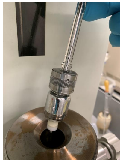
Figure 12: Transfer of mercury injected sample from low-pressure to high-pressure device.
