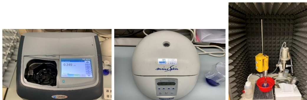
Figure 4: Required measurement devices for CEC determination. Left: Spectral-Photometer DR 6000 by Hach Lange, middle: Eppendorf MiniSpin centrifuge, right: ultrasonic UP 200H.
