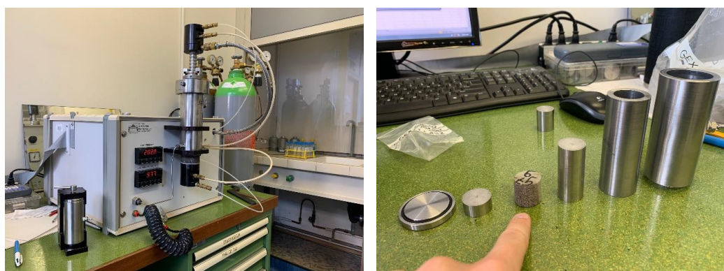
Figure 8: Left: AP-608 Automated Permeameter & Porosimeter machine with attached gas bottles (N, He) in the back and grain volume chamber in the front, right: close-up of grain volume chamber and calibrated metal blocks plus sample (pointed finger).
