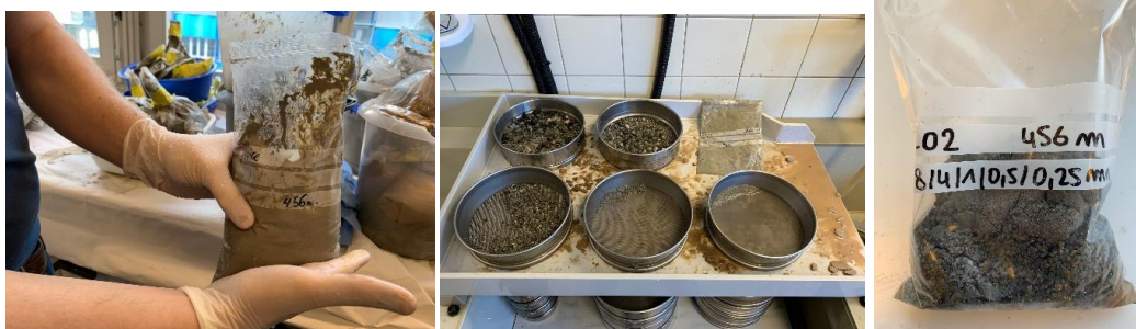
Figure 2: Washing and sieving steps of well cutting samples. Left: original sample as received from well site, middle: different mesh sizes of 8, 4, 1, 0.5 and 0.25 mm after washing, right: final, washed sample to be further dried in a 45°C oven.
