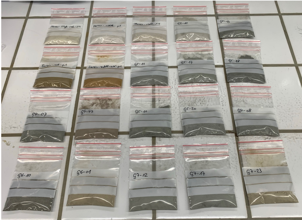
Fig. 3.9: Selected samples with fraction >400 \mu\text{m} of the glaciogenic deposits, Molasse Rouge, and Siderolithic formations as prepared for consecutive physico-chemical analyses. Note their different colours depending on type and amount of clay minerals.
