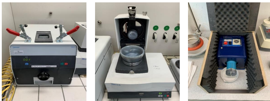
Figure 1: Overview of mills used for sample preparation. Left: jaw crusher for fraction <400 µm, middle: agate mill for fraction <63 µm, right: vibrating McCrone mill for fraction <20 µm.
