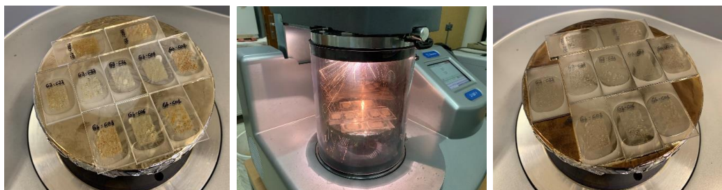
Figure 6: Carbon-coating of thin sections as prerequisite for QEMSCAN measurements. Left: thin sections without carbon-coating, middle: vaporizing graphite element, right: final carbon-coated samples.
