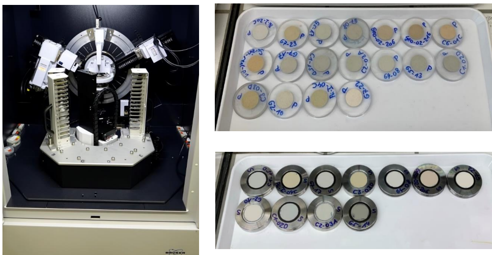
Figure 7: Left: XRD-device, right top: Powder (XRD-P) samples used for bulk analysis (Rietveld), right bottom: textured (XRD-S) samples used for clay mineral identification.
