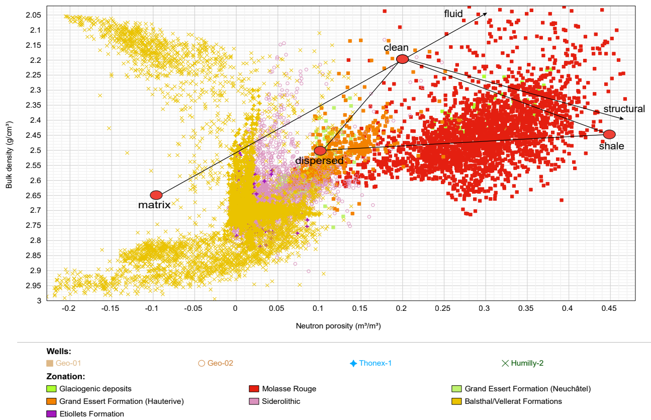
Fig. 5.3: Clay-type derivation using a Thomas-Stieber plot for eight formations. A trend towards dispersed shale is distinguished for the Hauterive Member of the Grand Essert Formation. Clay distribution for the Molasse Rouge ranges between the structural and dispersed types. After Haas et al. (2022).
