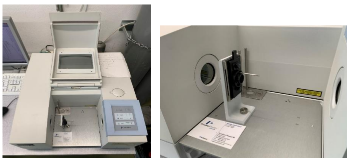
Figure 6: Left: Perkin Elmer Spectrum One FTIR device used for analysis, right: close-up of sample holder inside the measuring device when turned
