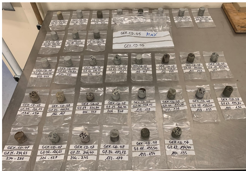
Fig. 3.8: Exemplified overview of drilled plugs on which petrophysical, geomechanical, geochemical, mineralogical and physico-chemical analyses were performed.
