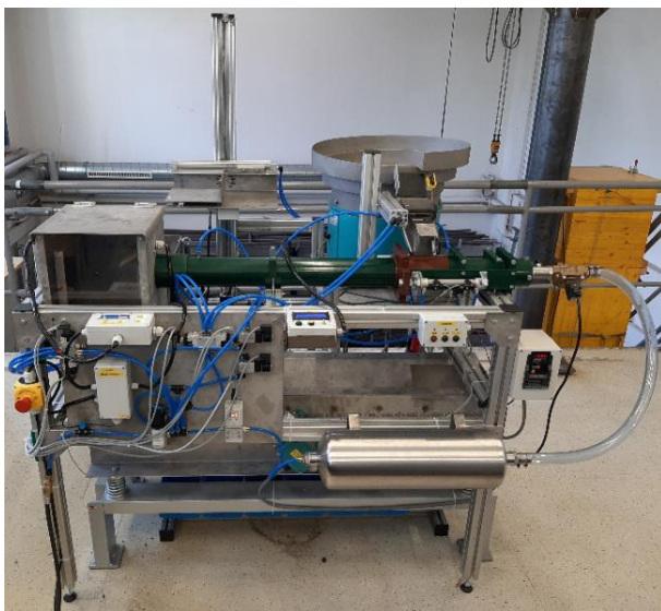
Figure 1. Automated single-particle impact tester
