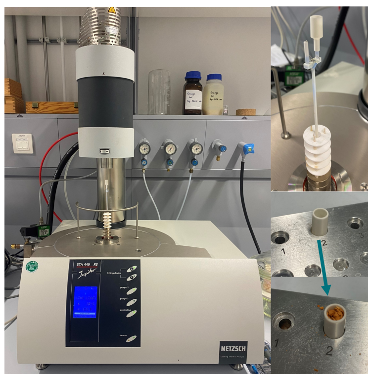
Figure 4.5: TGA setup and filling of ceramic pot
