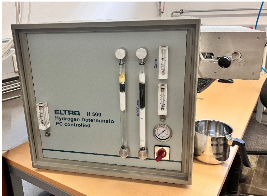
Figure 38. ELTRA H-500 analyser for residual hydrogen content measurements
