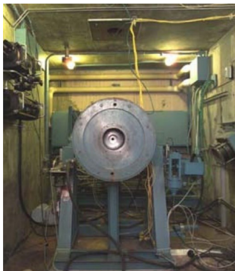
Figure 26. High-pressure testing rig up to 120,000 PSI and 1000°C [57]
