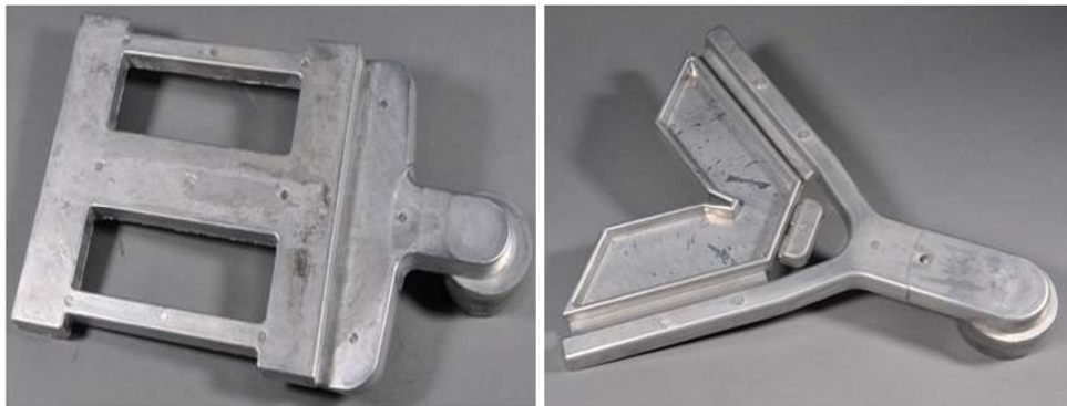
Figure 1. Stress lattice (left) and V-shaped (right) casting produced by high-pressure die-casting.
