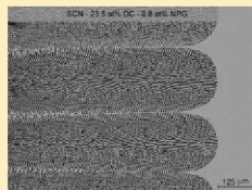
"Formation of eutectic cells in thin, polycrystalline samples from ternary organic SCN-DC-NPG alloys". In the presence of a third alloying element (NPG) the eutectic solid / liquid interface, composed of SCN and DC growing from the liquid, is constitutionally supercooled and subject to a complex sequence of instabilities that lead to cell formation. SCN: Saccharin, DC: D-Camphor, NPG: Neopentylglycol Courtesy: ACCESS e.V.
