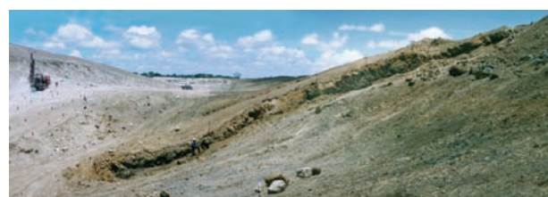
Figure 2—Trial mining of MSZ oxide ores at Hartley Mine, ca. 1998, view south. Note flat dip of the oxidized MSZ (brownish, approx. 2 m wide layer) towards the east (left side of photo)
