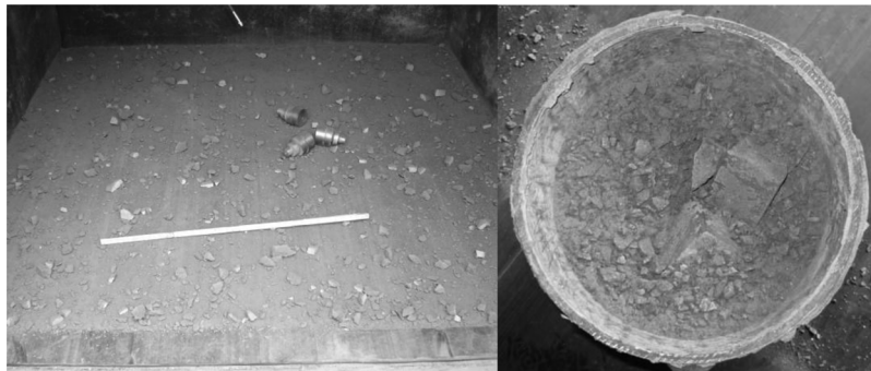
Figure 6 To the left: example of free face shots after blast. To the right: example of confined shots after blast
