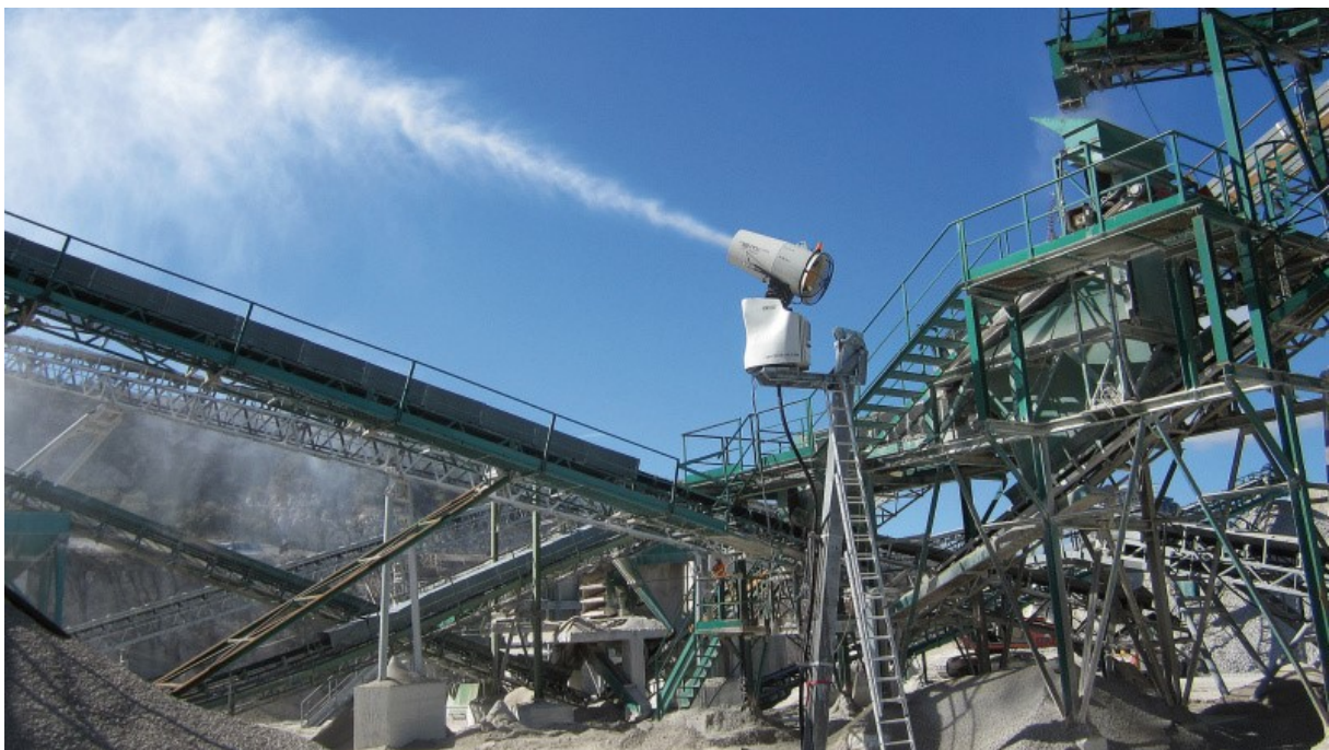
Figure 5-4: Dust suppression on conveyor belt [18]
