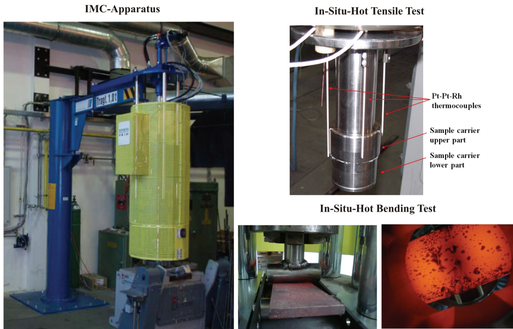
Figure 2. The IMC apparatus (left picture) which allows two different in-situ testing procedures (right pictures): the in-situ tensile test and the in-situ bending test.
