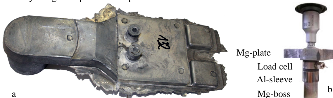
Figure 1: Reference part (a), bolted joint for relaxation tests (b)
