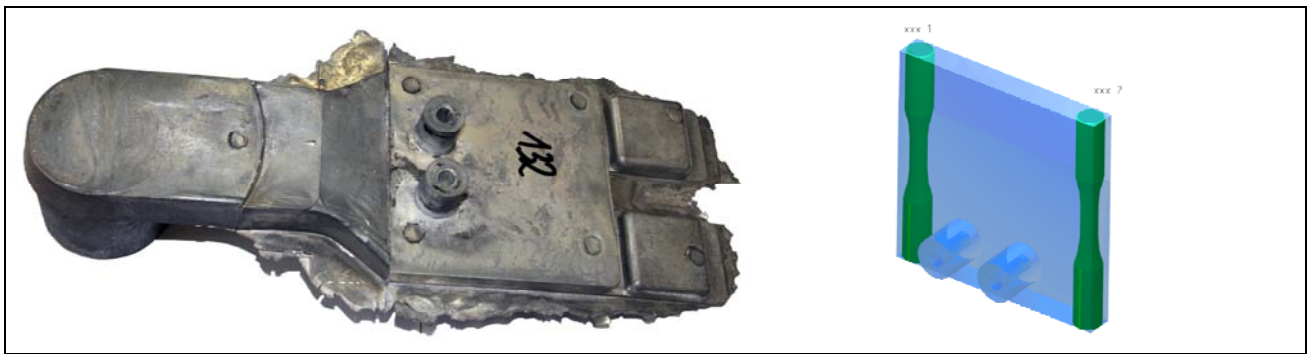
Figure 1: Die cast samples with gate system (a); position of specimen taking for creep tests (b) The chemical composition of the two investigated high pressure die cast alloys is listed in table 1.
