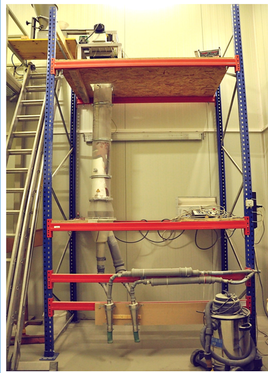
A prototype of the coaxial triboelectrostatic separator [8]
